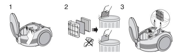
**NOTE** : Do not allow the filter to become clogged as this may cause power reduction or may damage the motor.
