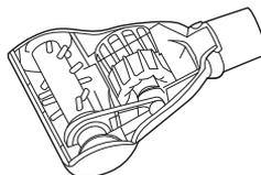
**NOTE:** When using the turbo brush, a loud noise can occur as a result of the high speed of the brush. This is normal.
