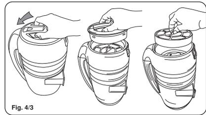
5. Hold the protective motor filter together with the holder over a dustbin. Only then should you separate both parts from each other. For a rough clean, Gently knock both parts over a dustbin.
