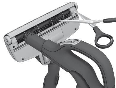
Disconnect the nozzle from the vacuum cleaner tube and remove entangled threads, etc. by snipping them off with scissors. Use the hose handle to clean the nozzle.
