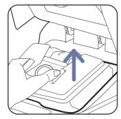
When the bag full indicator is red, the bag is full or blocked with dust particles. If the indicator remains red with the nozzle lifted off the ground, change the bag.
