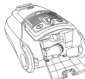
d. For washing the filters, please wash them in clean water, vibrate the filters to eliminate excessive water, then put them at a shady or cool place for air-drying. Please assemble them to the vacuum cleaner for using after they are completely dry, otherwise the motor will be damaged.
