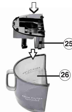
**Tips for assemble:** When assemble the cover back to the water container (26) after cleaning, please keep the dust container part (25) outside the water container.
